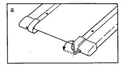
b. If the walking belt has shifted to the right, first remove the key and UNPLUG THE POWER CORD. Using the allen wrench, turn the right adjustment bolt clockwise 1/4 of a turn. Plug in the power cord, insert the key and run the treadmill for a few minutes. Repeat until the walking belt is centered.
